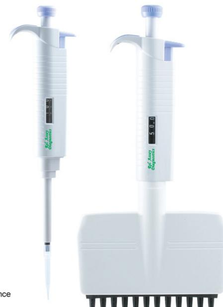
**Note:** It is recommended to check the performance of the pipette after each autoclaving. It is also recommended to grease the piston and seal of the pipette after each 10 autoclaving.
